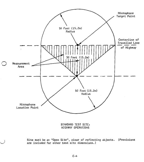
Test Site: Test site should conform to dimensions indicated in the figure below:
